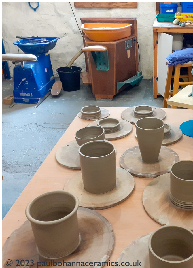
Wheel-thrown parts drying a little before turning and assembling into bigger pots.
